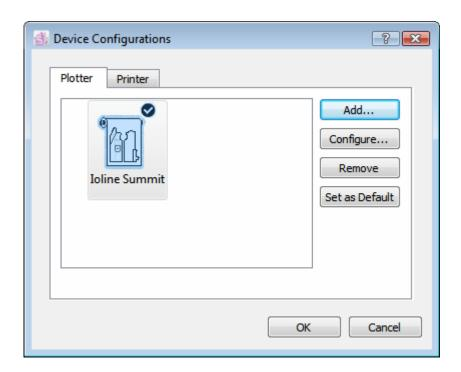
**Configure...:** Change the setting of the selected driver. Click *Configure...* or double click the mouse button on selected driver to change the setting or the driver of existing Plotter.
